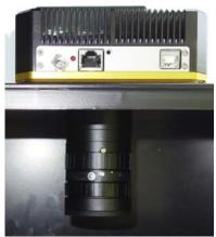
The CCD unit can be removed after first unscrewing the lens (left) to reveal three M3 bolts (right), which can then be unscrewed. There is no seal between the CCD unit and the box, and no adjustments, so the CCD unit can be easily replaced. Do not touch the exposed surfaces of the CCD cover glass or lens, the front of which is protected by a UV filter.
